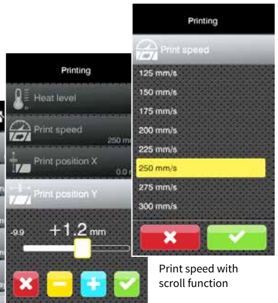
Print position Y slide control for fast adjustment ± keys for fine adjustment
